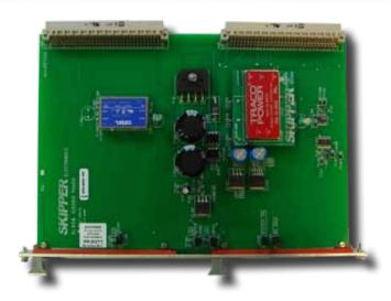
The PP-D271 is a PCB Tranceiver power for the SKIPPER DL850 Navigational Speed Log.
